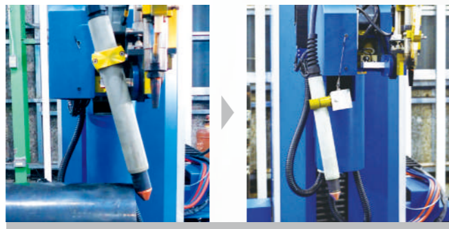
Magnetic torch protection [ Break-away torch system ]
