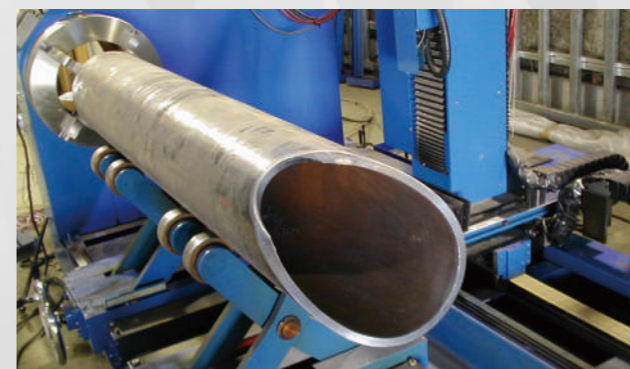
Cutting with AWS Intersecting angle of 37 degrees
