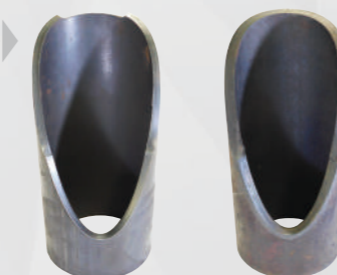
TOKYO SKYTREE Welding preparation (Upper part)
