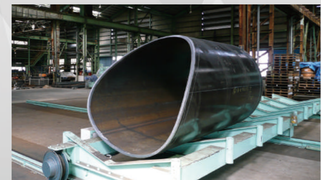
Cutting piece with 4 reference line marking
