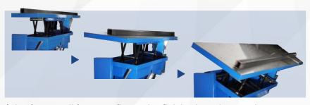
It is also possible to configure the finished products to be automatically ejected.
